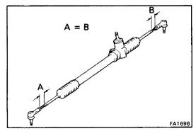
If wheel angles differ from the standard specifications, check to see if the lengths of the left and right tie rods are the same.
