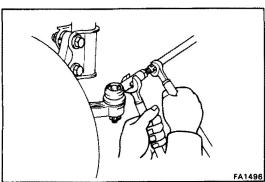
(h) Adjust toe-in by turning the left and right rack ends an equal amount.
