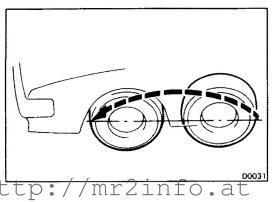
(d) Advance the vehicle until the marks on the rear sides of the tires come to the measuring heights of the gauge on the front side.
