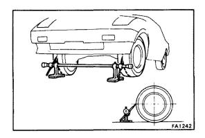
(e) Measure the distance between the marks on the front of the tires.
