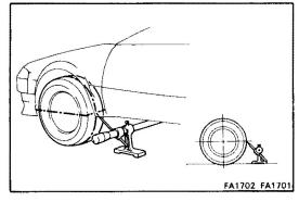
(c) Mark the center of each rear tread and measure the distance between the marks of the right and left tires.
