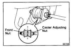
If caster is not within specification, adjust by turning the nut.
