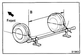
(d) Advance the vehicle until the marks on the rear sides of the tires come to the measuring heights of the gauge on the front side.
