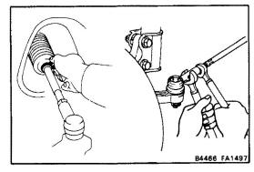
(g) Remove the boot clips and loosen the tie rod lock nuts.
