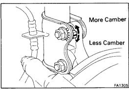
If camber is not within specification, adjust by turning the camber adjusting cam.
