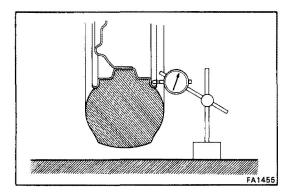
(b) Check the wheel runout.
